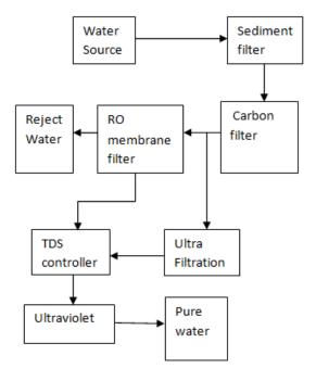
Figure 1. Schematic diagram of the stages in Reverse Osmosis
