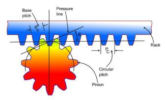
Figure 2.1. Rack and pinion
