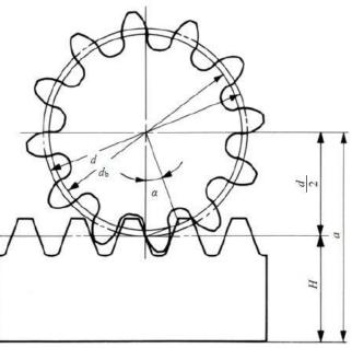
Figure 2.2. Rack and pinion
