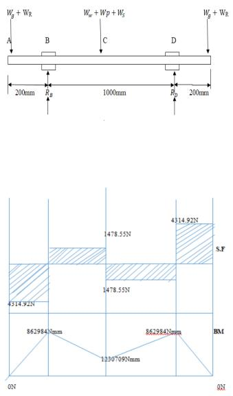
**Figure 2.4.** Shear Force And Bending Moment Diagram Of The Shaft.
