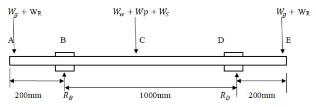
Figure 2.3. The bending moment on the shaft
