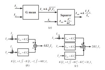
Figure. 1. Block diagram of the proposed multiplier [16]
