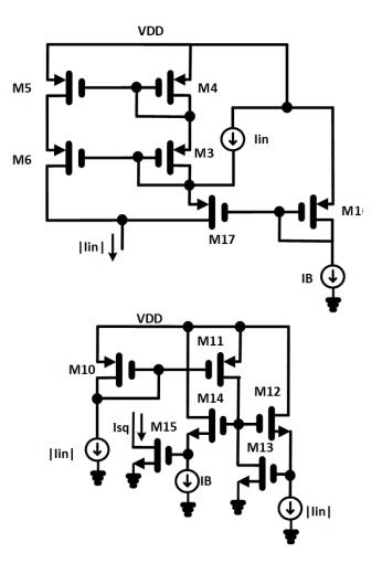
Figure. 3. The squarer with the absolute-value circuit
