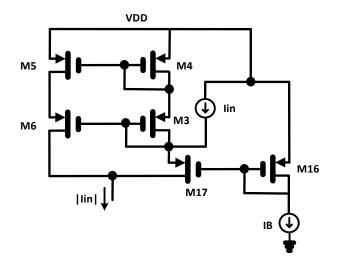
Figure. 2. Absolute-value circuit of the RMS-to-DC converter.
