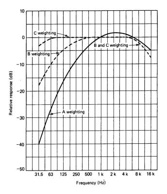
Figure 1: Frequency response for the A, B & C weighting networks
