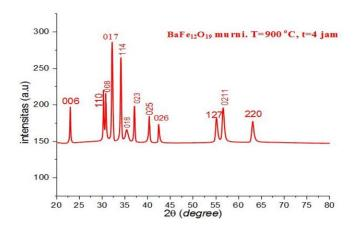
Figure 1. XRD pattern of BaFe<sub>12</sub>O<sub>19</sub> (matrix)
