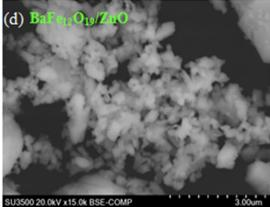
**Figure 5.** Scanning Electron Microscope results of BaFe<sub>12</sub>O<sub>19</sub> and BaFe<sub>12</sub>O<sub>19</sub>/ ZnO
