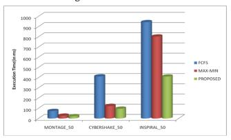
Fig.4.2 : Makespan Comparison of Scheduling Algorithms for VM=30.
