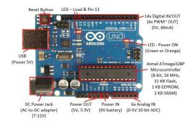
Figure 8. Arduino Board.
