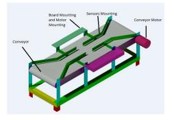
Figure10. Conveyer Belt with separation tray.
