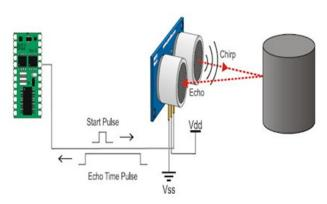
Figure 6. Working of Ultrasonic Sensor.
