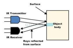
Figure 3. Working of IR Sensors.
