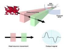
Figure 4. Working of PIR Sensor
