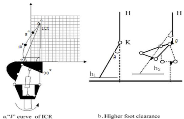
Fig 8. Advantages of 4-bar knee joint
