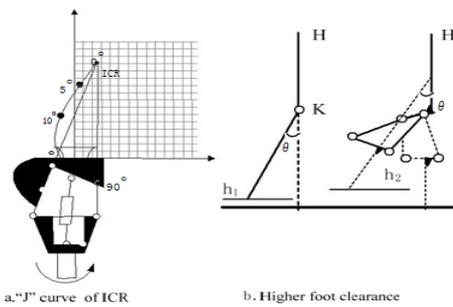
Fig 5. Advantages of 4-bar knee joint
