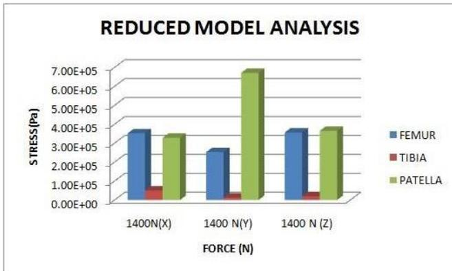
**Fig 11** : Reduced model stress analysis
