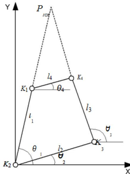
Fig.7 Schematic diagram of 4-bar closed-chain knee mechanism
