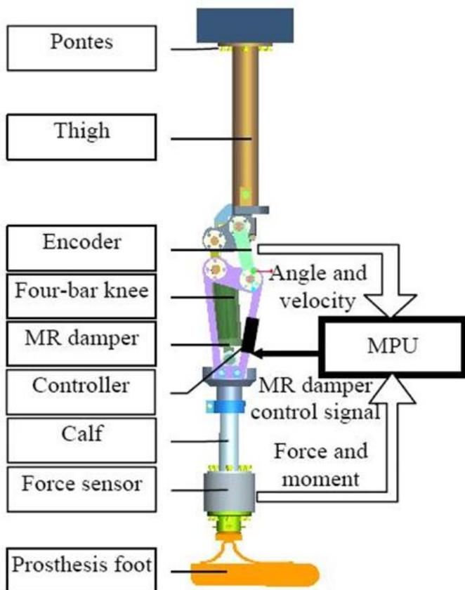
Fig. 2 Virtual prototype of IBL
