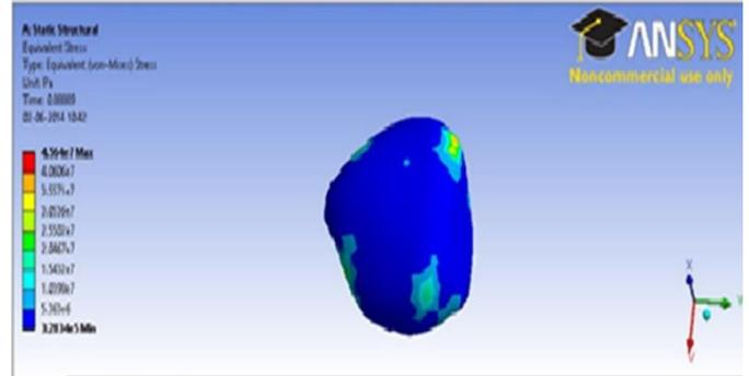
Fig 10.C (TIBIA) model analysis of knee joint
