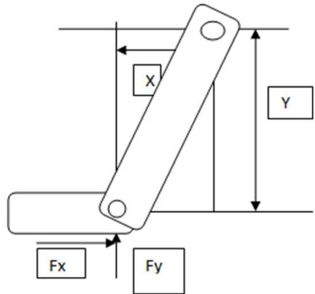
**Fig 9.** Forces applied to the knee joint
