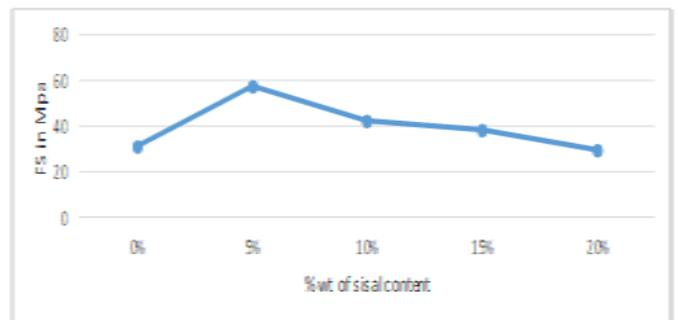
Figure 10: Graph 3: % wt of sisal vs Flexural strength
