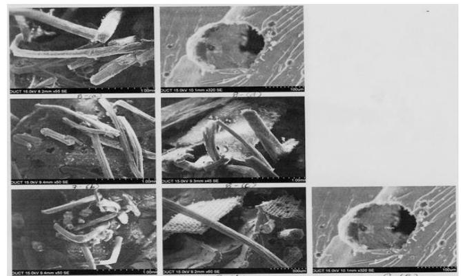
Fig. 14. SEM images of (a, b) are the 3% of Carbon and glass fiber + 17% of sisal fiber + 80% of resin; (c, d, e, f, g): are the 5% of Carbon and glass fiber + 15% of sisal + 80% of resin.
