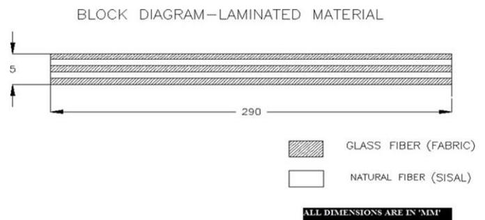
Figure 6: Block diagram of laminated material
