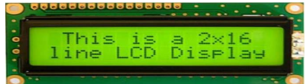
Figure 4 : LCD screen used to Display Text
