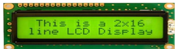
Figure 4 : LCD screen used to Display Text
