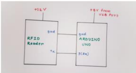
Fig 2. Interfacing RFID with Arduino
