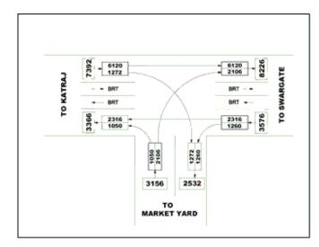
**Figure 4 :** Traffic flow diagram of Utsav Intersection during morning peak
