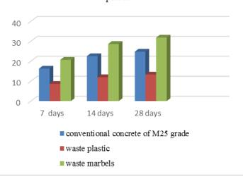
Graph 1. Comparison between conventional concreteM25 grade with Waste marble and Waste plastic
