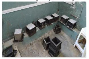
Figure 1. Casting of cubes Table 7. Comparison between Conventional concrete with replacement of course aggregate (waste marble and waste plastic)
