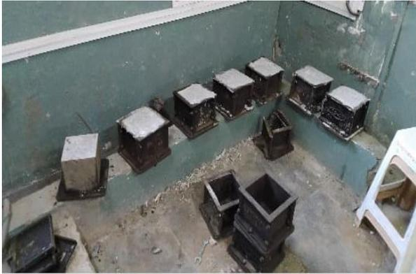
Figure 1. Casting of cubes
