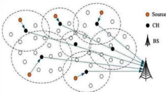
**Figure 1.** Basic Architecture for Wireless Sensor Network Correspondence area and partitioning of base stations are genuine stresses that must be considered when performing grouping of remote sensors. The correspondence between the bunch head
