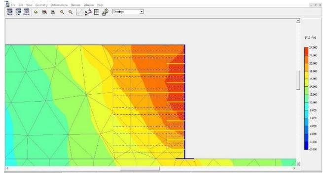
Figure 8. Maximum deformation at top of wall
