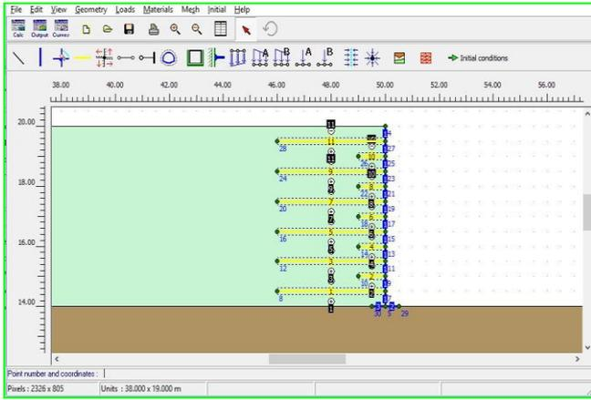
Figure 5. Geometric model of RE wall
