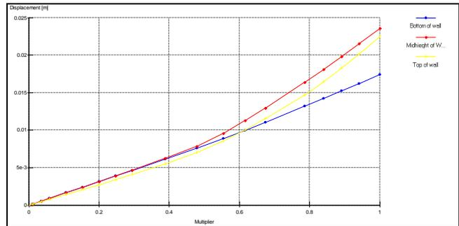
Figure 9. Deflection at different points on wall
