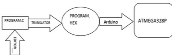
Fig.4 Device Programming
