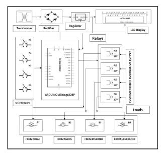
Fig.1 Block Diagram Auto Power Supply
