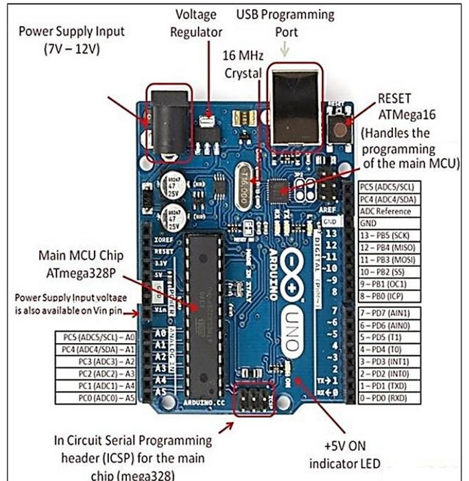
Fig.2 Pin diagram of ARDUINO.
