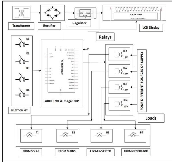
Fig.1 Block Diagram Auto Power Supply
