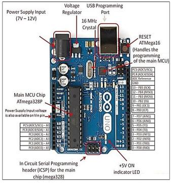
Fig.2 Pin diagram of ARDUINO.
