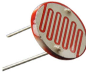
Fig.4: Light Dependent Resistor (LDR)
