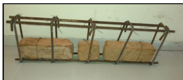
Photo 3. Cage of brick in filled beams section
