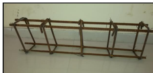
Photo 2. Cage of conventional beam setion
