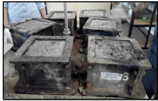
Photo 6. Compaction of cubes
