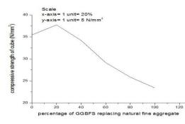
Figure 1: Variation between cube compressive Strength and percentage of GGBFS replacing natural fine aggregate
