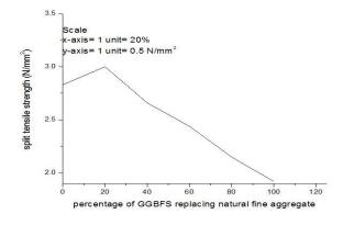
Figure 3: Variation between split tensile strength and percentage of GGBFS replacing natural fine aggregate
