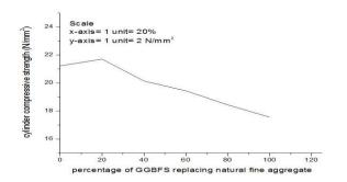
Figure 2: Variation between cylinder compressive Strength and percentage of GGBFS replacing natural fine aggregate
