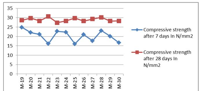
**Graph. 3.0.** Compressive strength results of Fly-ash, metakaoline and steel dust in concrete
