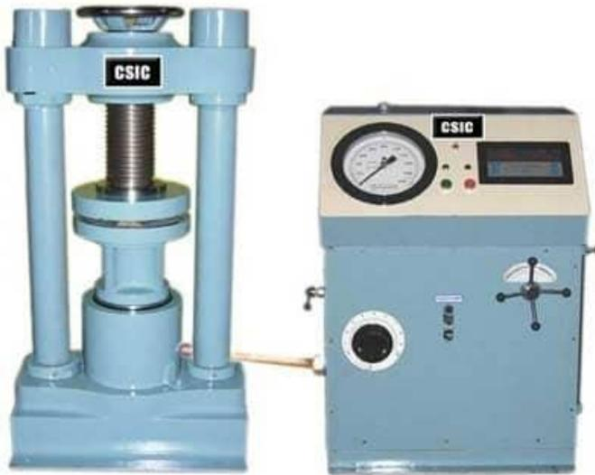
Figure 1. compressive testing machine
