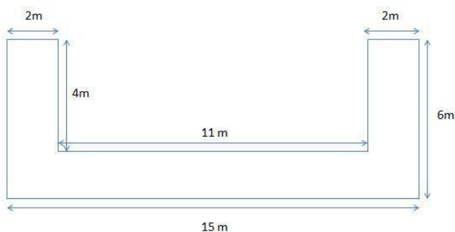
Fig 1: Schematic diagram of the hearth used in the study
