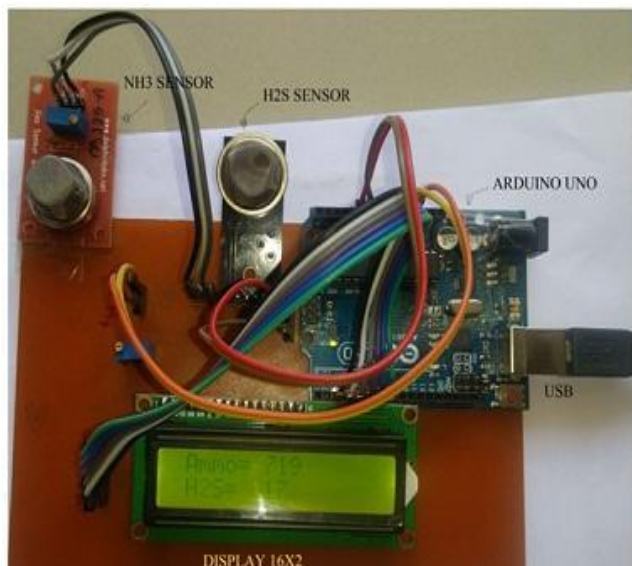
Fig.1 Arduino Uno based odor sensory measurement system
