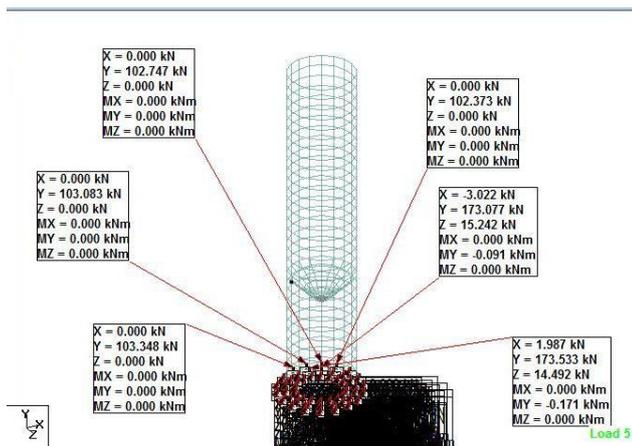
From above manual calculation it is found that wall of silos required 2.81 % of steel on wall to resist pressure due to grain.
