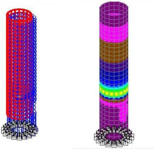
Thickness of wall is 150mm. 8 m high silo supported with 4 column designed for fill condition. Pressure of wheat is considered to calculate pressure on wall of silo
