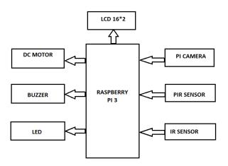
Fig-1: Block diagram of proposed work
