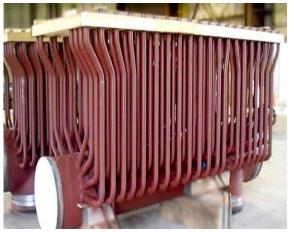
The modification of front wall tubs headers that the addition of tubes to increase the area so that the increasing in the boiler efficiency. The Increases the area to increasing the boilers efficiency. E.g. the old tube size is 76.2OD\*4.06\*12525 and new tubes size is 76.2OD\*4.06\*13129.when the area increasing to increase the boilers efficiency. The heating area increasing this condition to increasing efficiency by 2.08%
