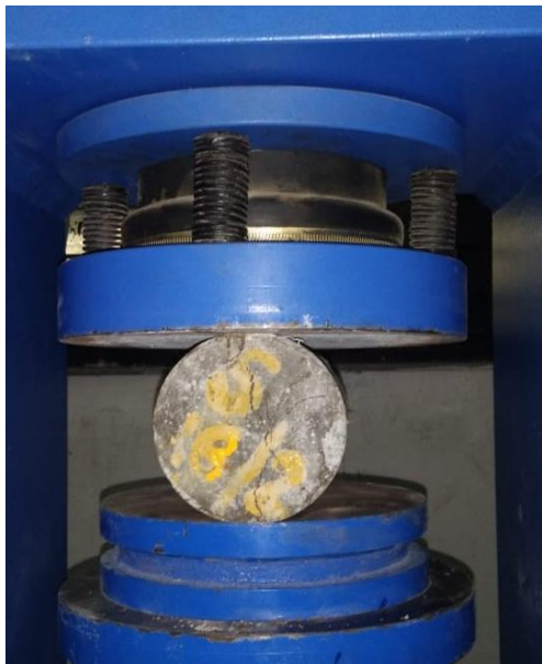
Fig – 2.2 Split tensile strength test
