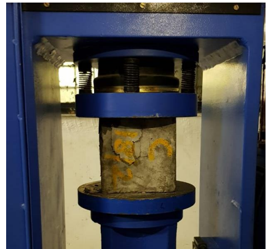
Fig – 2.1 Compressive strength test
