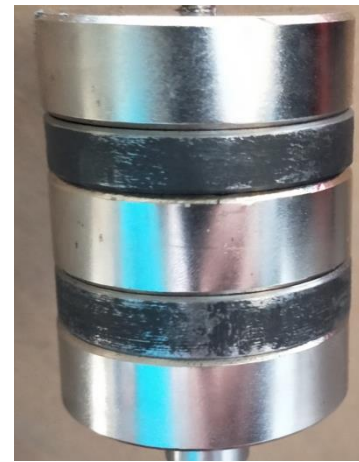
Figure 4. Set of Magnet and iron core We used N45 neodymium Magnets.
