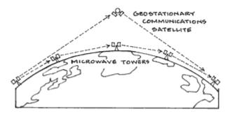
dissipate into the ocean. Over short distances, we erect microwave towers every 25 miles or so to act as "repeaters" to repeat and boost the signal. Think of a geostationary communications satellite as a repeater in the sky.
