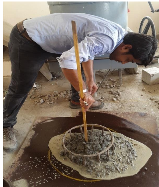
Fig. 4.11: Performing Slump Flow/J-Ring combination test
