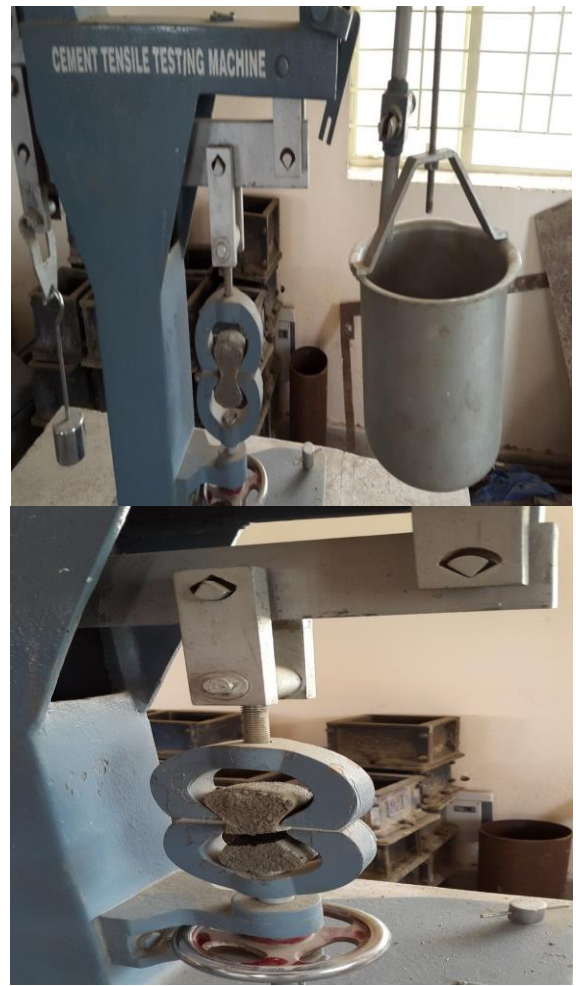
Fig. 4.4: Performing tensile strength test for 28 days
