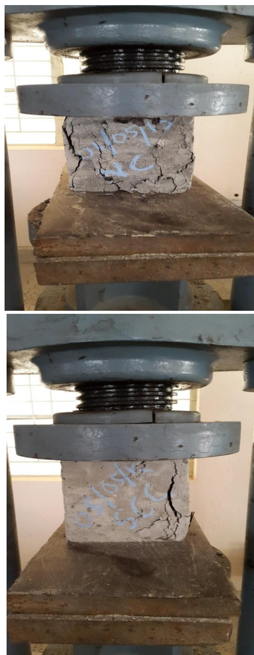
Fig. 4.1: Performing compressive strength test for 28 days
