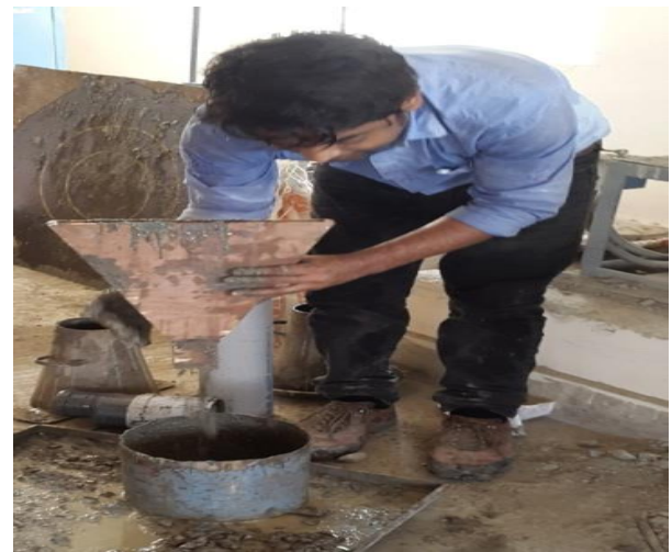
Fig. 4.9 : Performing Orimet Test (Flow Time in second) and V-funnel test
