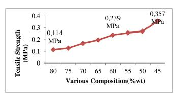
**Figure 6** Test Results of Biofoam Tensile Strength Based on Leaves and PVAc at Various Variations in Composition,
