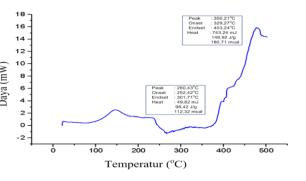
Figure 9 : Thermal Analysis (DSC) of Biofoam Materials in Composition Variations of 80% wt.
