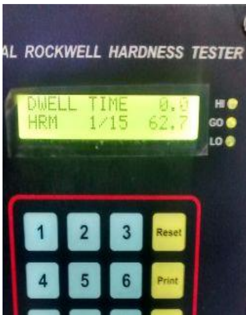
Fig.17 – Hardness Test Reading
