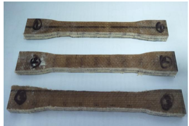
Fig.13(a)- Tensile Specimen before Fracture
