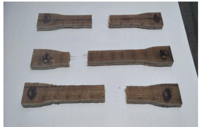
Fig.13(b) – Tensile Specimen after Fracture
