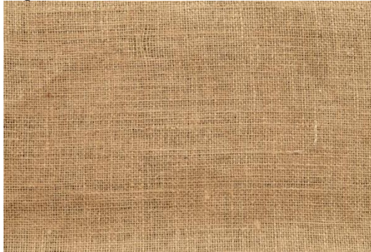
Fig.2 – Flax Mat(0 0 / 90 0 orientation)
