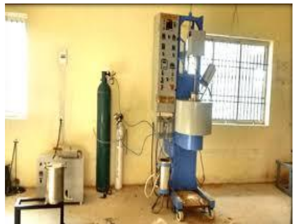
Fig 4: A stir casting setup as shown in Figure, consist of a Coke fired Furnace and a stirrer assembly, which was used to synthesize the composite.
