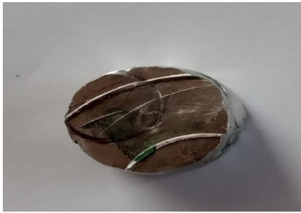
Fig 10: Compression Specimen after the test.
