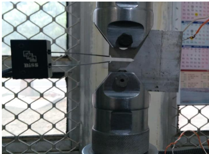
Fig. 4. – Specimen gripped on fatigue testing machine
