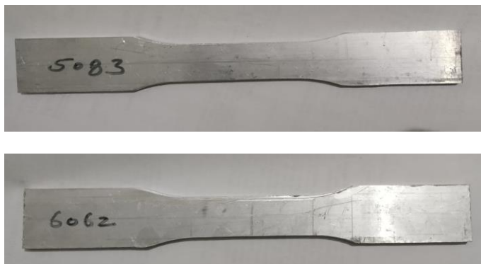
Fig 1- Specimen of AA 5083 and AA 6062 for tensile testing
