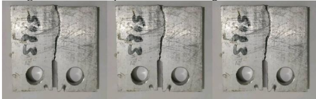
Fig 5 - Fractured specimens after fatigue test AA 6062
