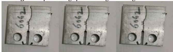
Fig 5 - Fractured specimens after fatigue test AA 6062
