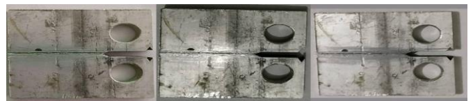
Fig 7. Fatigue growth test CT specimen.
