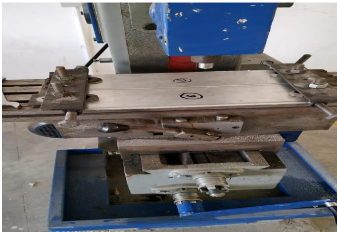
Fig 2. Friction Stir Welding (FSW) Setup
