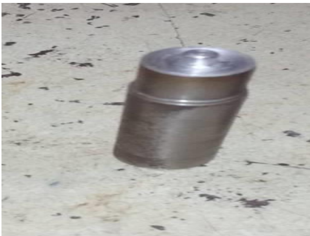
Fig. 3. Tool used for FSW with 24mm shoulder diameter and 5mm pin length.
