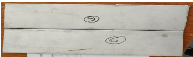
Fig .4. Plates of AA 5083 and AA 6062 before joining.
