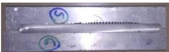
Fig 5. Plates of AA 5083 and AA 6062 after joining.
