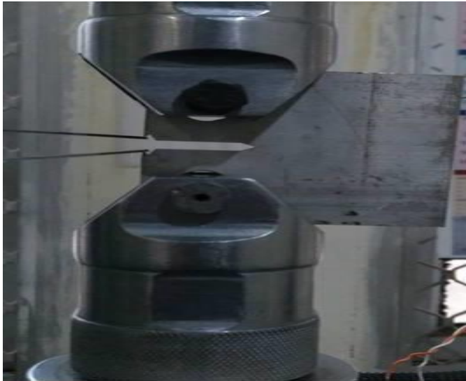
Fig. 8. – CT Specimen gripped on fatigue testing machine
