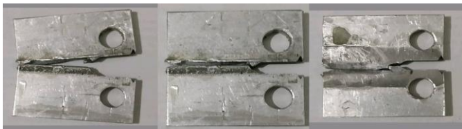
Fig 9. Fractured CT specimens after fatigue test.
