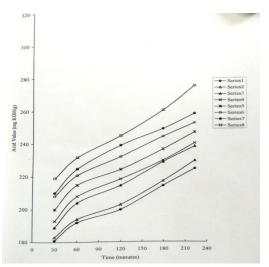
**Fig.2** Change in Acid Value during Maleinization of Rice Bran Fatty Acids
