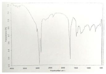
Fig 5. FTIR spectrum of Pure Rice bran Fatty Acids
