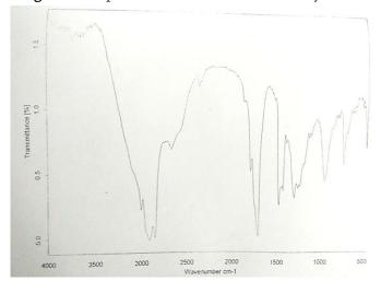
**Fig 6.** FTIR spectrum of Maleinized Rice bran Fatty
