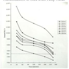
**Fig. 3.** Change in Unreacted Maleic Anhydride during Maleinization of Rice Bran Fatty Acids
