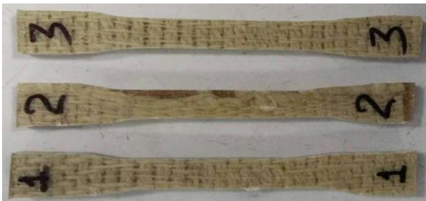
Figure 9(a)-Tensile Specimen before Fracture
