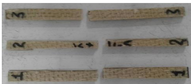
Figure 12(b)-Flexural Specimen after Fracture
