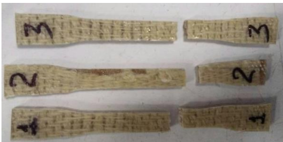
Figure 9(b)-Tensile Specimen after Fracture
