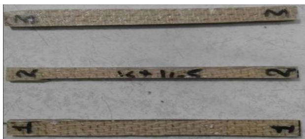
Figure 12(a)-Flexural Specimen before Fracture
