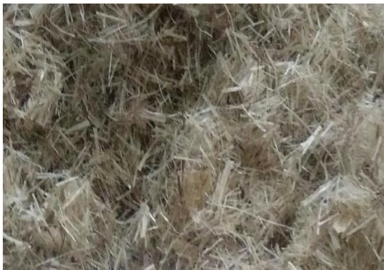
Figure 2 (b)- Hemp fibre after cutting
