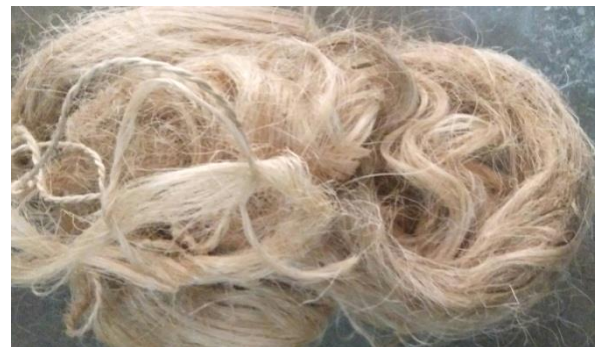
Figure 1(a)- Banana fibre before cutting
