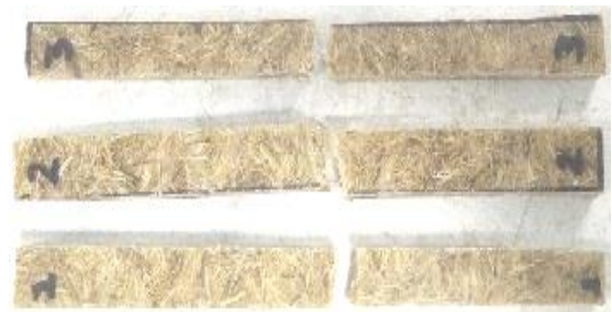
Figure 13(b)- Flexural Specimen after Fracture
