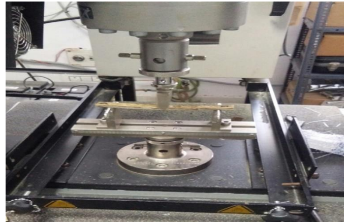
Figure 12- Flexural specimen fixed in UTM vice
