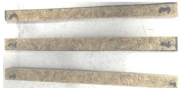
Figure 13(a)-Flexural specimen before fracture
