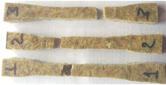
Figure 10(b)-Tensile Specimen after Fracture
