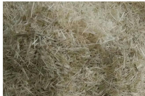
Figure 3(b)- Sisal fibre After cutting
