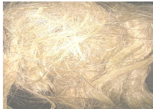
Figure 3(a)- Sisal Fibre before cutting
