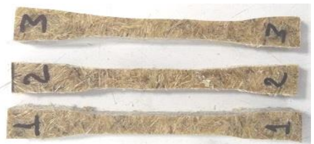
Figure 10(a)- Tensile Specimen before Fracture
