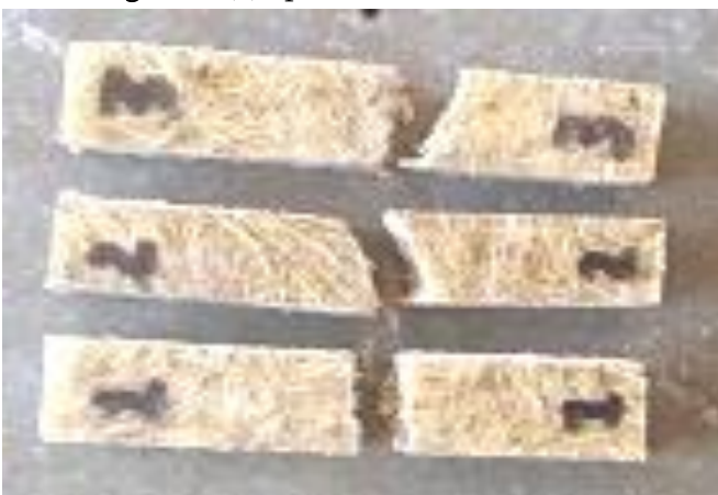
Figure 10(b)- specimen after fracture
