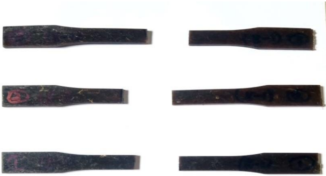
Fig 6(b)- Tensile specimen after fracture (Batch 1)
