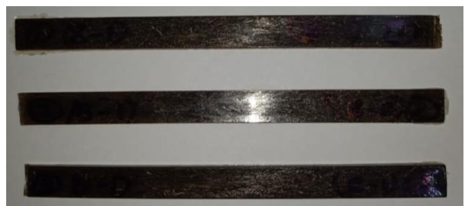
Fig 10(a)-Flexural specimen before fracture (Batch 1)
