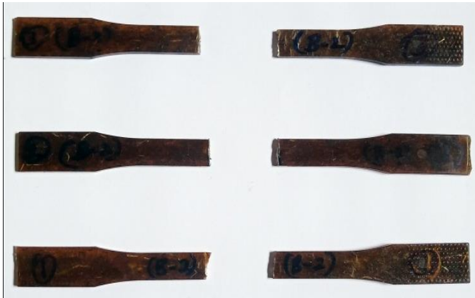
Fig 7(b)-Tensile specimen after fracture (Batch 2)
