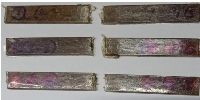
Fig 11(b)-Flexural specimen after fracture (Batch 2)
