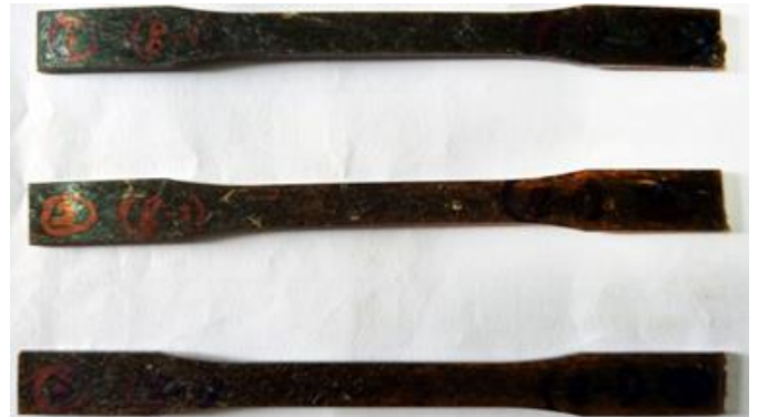
Fig 6 (a)- Tensile specimen before fracture (Batch 1)
