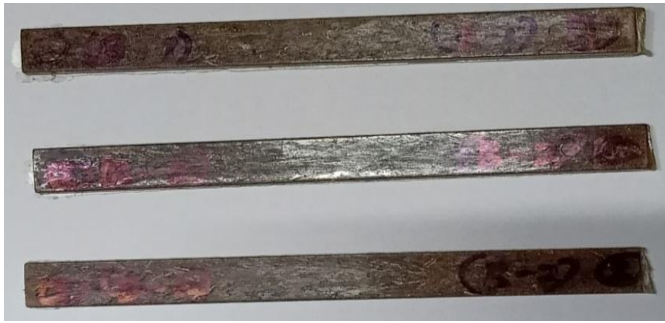
Fig 11(a)-Flexural specimen before fracture (Batch 2)
