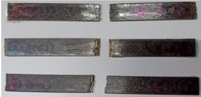
Fig 10(b)-Flexural specimen after fracture (Batch 1)
