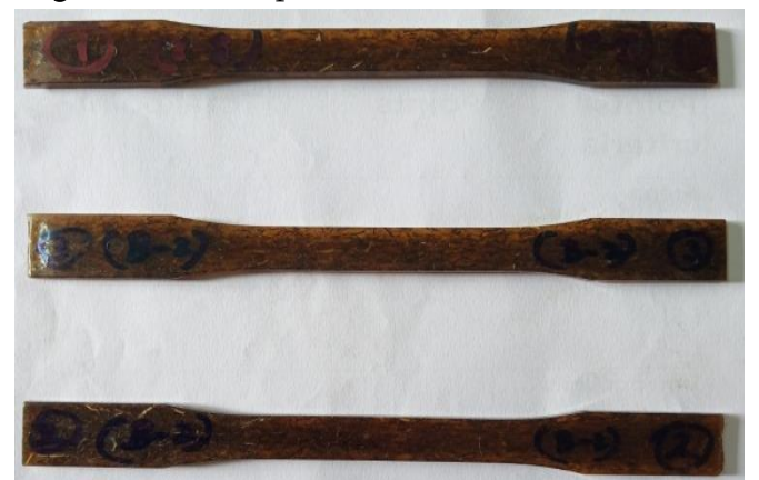
Fig 7(a)-Tensile specimen before fracture (Batch 2)
