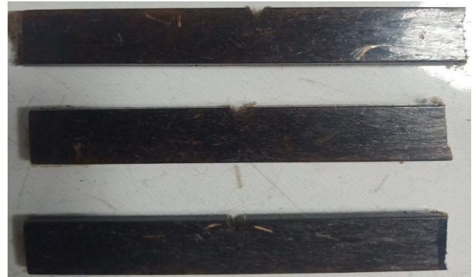
Fig 6 (a)- Impact specimen before fracture (Batch 1)
