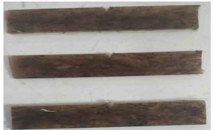
Fig 6(b)- Impact specimen after fracture (Batch 1)
