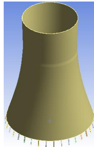
Figure 2. Cooling Tower with I support
