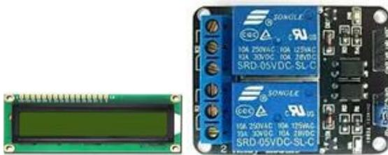
**Figure 3.** LCD display screen and 2 Channel Relay
