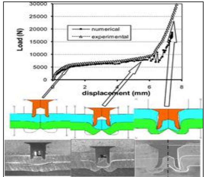
Fig 7. Deformed shape and load–displacement curve in the 2D FEM model
