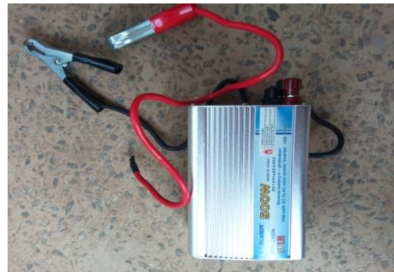
Figure 5. The 500W inverter and its connecting probes
