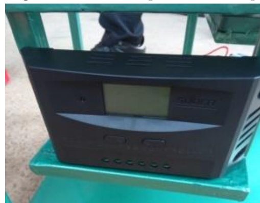
Figure 2. The charge controller
