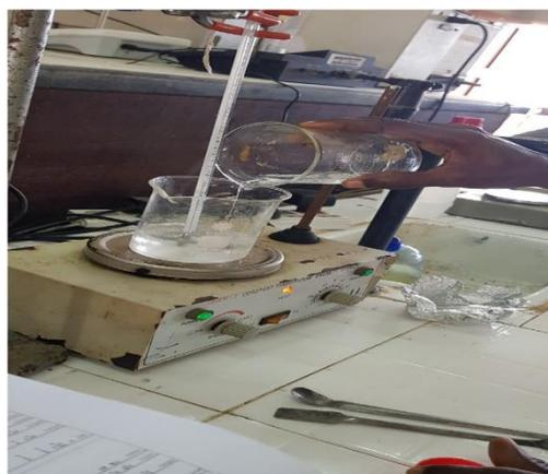
Figure 1 : The mixture (Calcium nitrate tetrahydrate and Magnesium nitrate hexahydrate) was placed on a magnetic stirrer and under continuous stirring and heating at 80 C<sup>o</sup>
