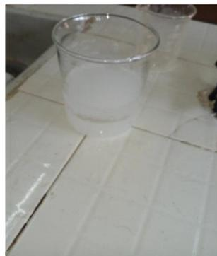
Figure 3: mixture of calcium nitrate tetrahydrate and magnesium nitrate hexahydrate
