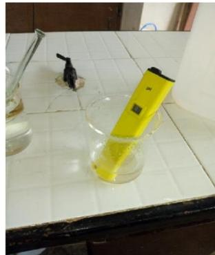
Figure 4: PH meter for adjusting the PH of the mixture to 8
