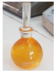
Figure 12: Specific Gravity Bottle with Oil
