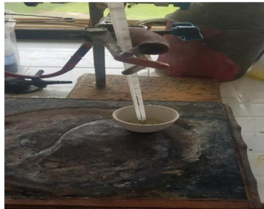
Figure 11: Set-up for determining smoke, flash, and fire points
