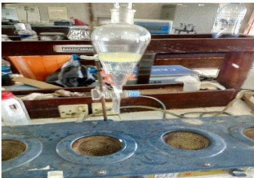
Figure 10: water (lower region) and biodiesel (upper region)
