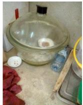
Figure 7: Storing the catalyst in the desiccator prior to use.
