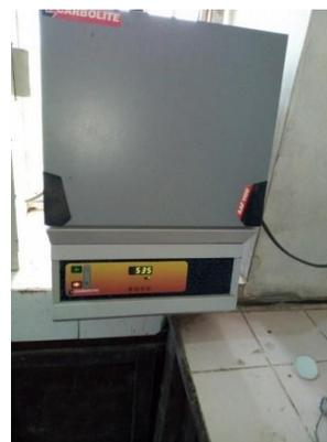
Figure 6: The precipitate calcined in the muffle furnace at temperature at temperature ranging from 550-600 C°
