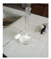
Figure 2: standard flask to prepare 0.1M of sodium carbonate (Na2CO3)
