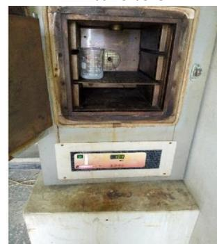
Figure 5: The precipitate stored in the oven at temperature 110 C overnight
