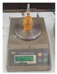
Figure 13: Measurement of SGB weight
