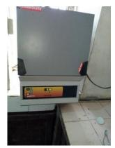
Figure 6: The precipate calcined in the muffle furnance at temperature at temperature ranging from  $550\text{-}600\ \text{C}^\circ$
