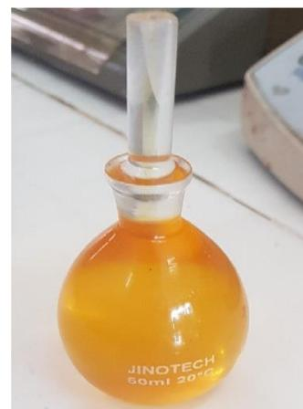
Figure 12: Specific Gravity Bottle with Oil
