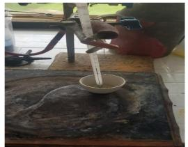
Figure 11: Set-up for determining smoke, flash, and fire points 2.7.4 Determination of Specific Gravity
