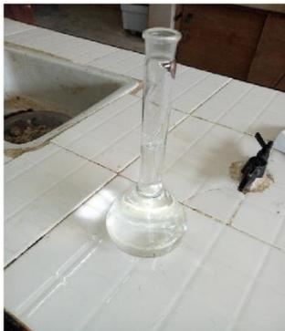
Figure 2: standard flask to prepare 0.1M of sodium carbonate ( $\text{Na}_2\text{CO}_3$ )
