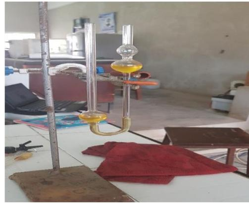
Figure 14: On-going viscosity test
