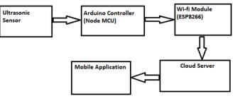
Figure 1. System Architecture
