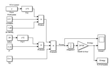
Figure 2: The Block diagram for wind Turbinr
