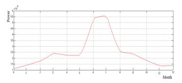
Figure 4: The output Power with month for wind turbine
