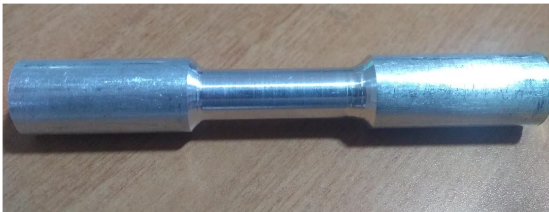
Fig.8 Aluminium Test specimen used for Testing.
