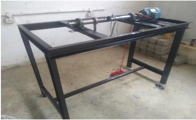
Fig.2 Rotating beam Cantilever Type Fatigue Testing Machine
