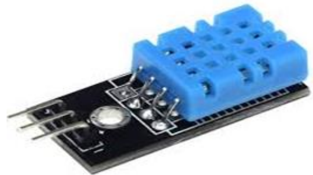
Figure 4 Temperature and Humidity sensor
